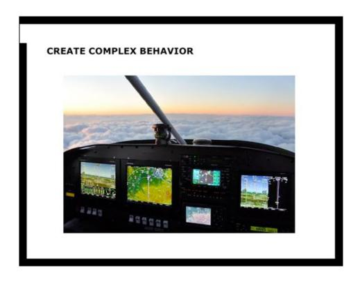
Information enables behavior that's orders of magnitude more complex than possible with just mechanics, at a fraction of the cost. This is a modern small airplane avionics system. It consists of a bunch of small fairly standard computers running special software.
