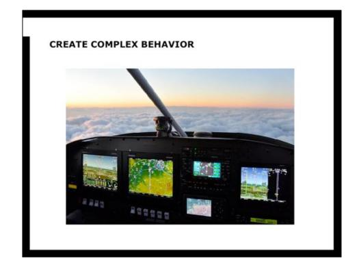
Information enables behavior that's orders of magnitude more complex than possible with just mechanics, but at a fraction of the cost. This is a modern small airplane avionics system. It consists of a bunch of small fairly standard computers running special software.
