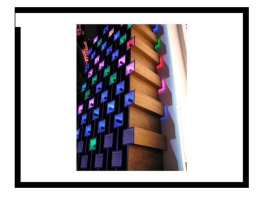
We also have bigger plans. Here's an RFID wine rack prototype we made for WIRED Magazine's NextFest in LA. In this rack, each bottle has an RFID tag on it, and there's a reader in every cell. The rack knows exactly which bottle is in which cell and projects different kinds of information directly onto the wine bottles.
