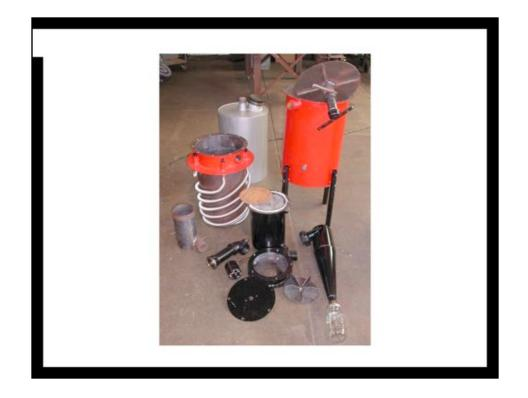
An alternative energy generator created by All Power Labs, another Bay Area company. It converts burned trash into a gas you can drive you car with. Their components are made of steel that has been cut using a computerized plasma cutter that costs about the same as the first LaserWriter. They have open sourced the design so that you can download the design and make your own generator if you have your own plasma cutter.
